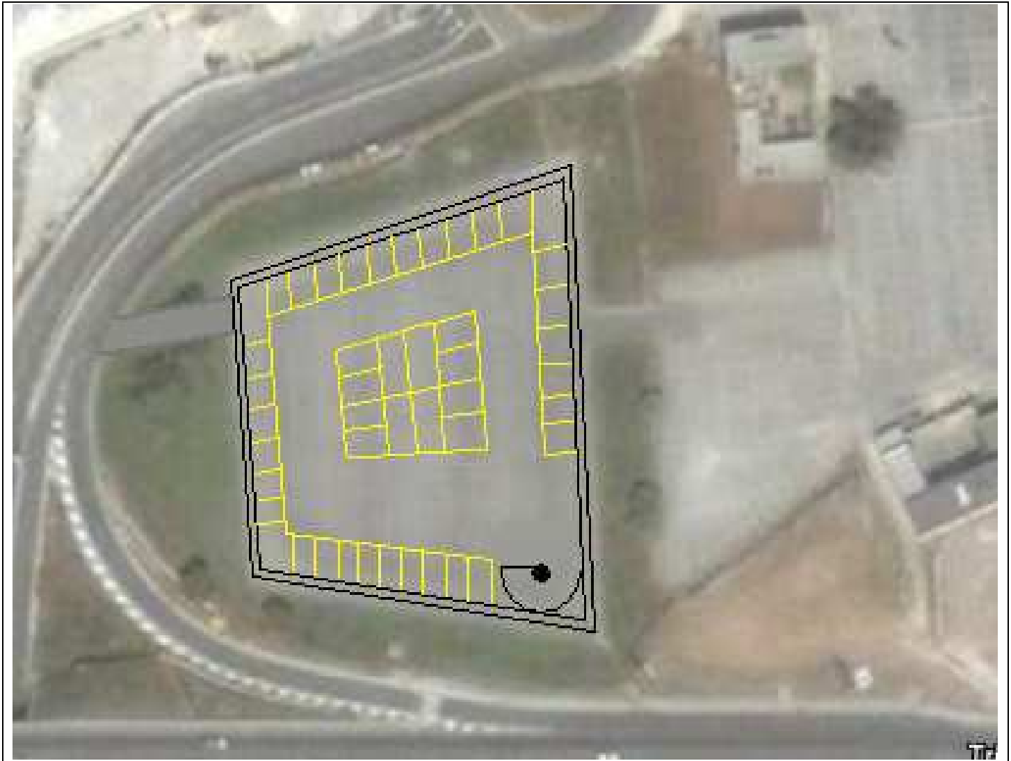
Plan view of the first floor of the proposed multi-storey car park
